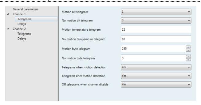
The configuration of the sensor behavior when there is a motion detection and when it finishes is done here. The working mode and parameterization of both channels is done in the same way and they have similar parameters that are explained next:
